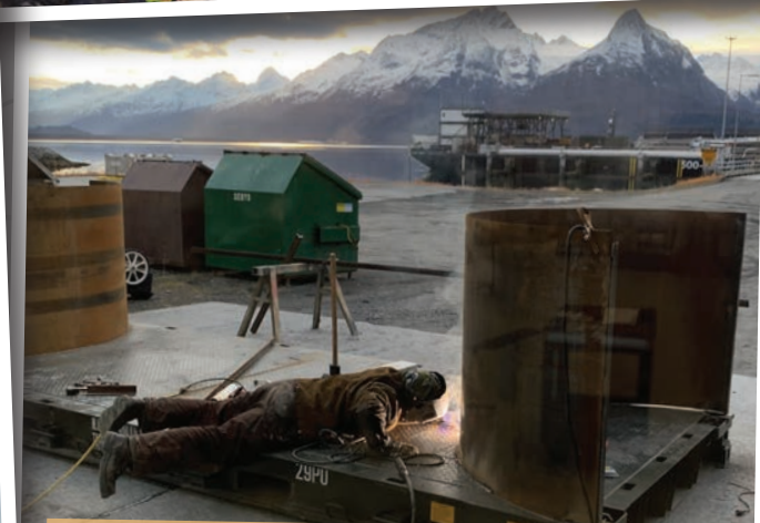
Local 302 mechanic and operator James Wiese welds fairleads onto a 20' flat for Tatitlek Chenega Chugach contract at Alyeska's Ship Escort Response Vessel System Base in Valdez, Alaska; These fairleads will assist in boom deployments and retrievals during sensitive area protection deployments at the Port of Valdez
