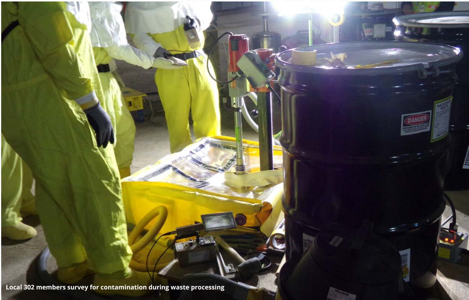
Local 302 members prepare transuranic and low-level waste to be shipped to the Waste Isolation Pilot Plant (WIPP) in New Mexico
