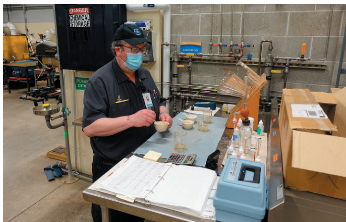
Jesse Figgins performing boiler chemistry at Swedish Issaquah Campus; checking conductivity and looking for adequate scale inhibitor and oxygen scavenger
