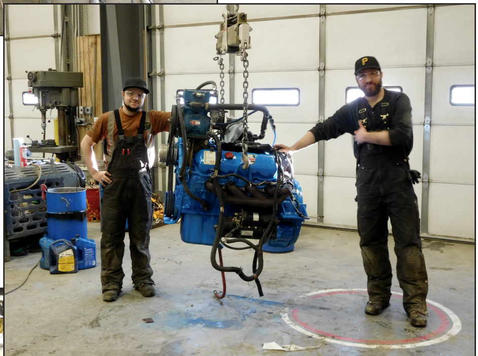
Apprentice mechanics Tim Craft and Connor Irvine show off their show-piece Detroit after head-gasket replacement and prepping it to go back in a Grove 760 crane
