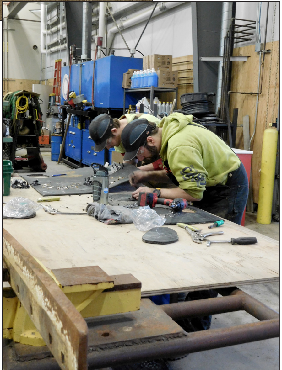
First year apprentice mechanics practice their ability to properly install conveyor belt patches
