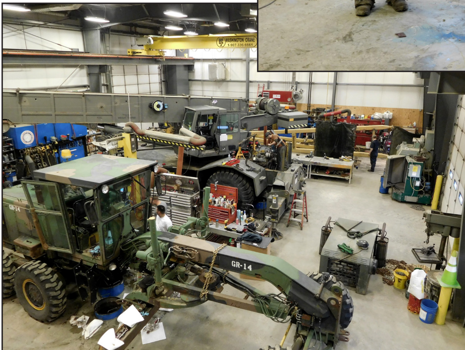
A busy shop; 130 Cat motor grader repair and maintenance, Grove 760 engine repair, and side boom line-boring all happening simultaneously
